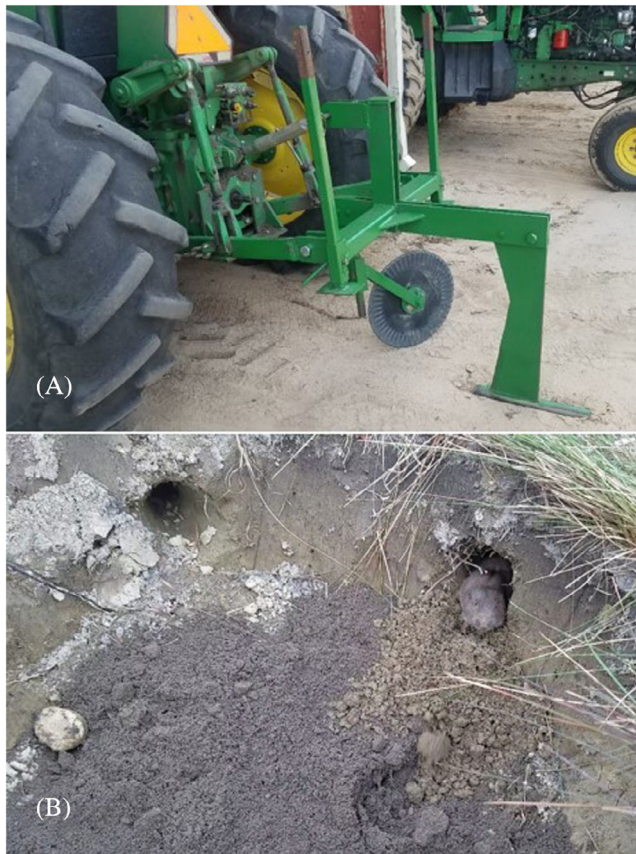
Figure 2. (A) Burrow building plow and (B) resulting burrow used in translocation of 15 southeastern pocket gophers ( Geomys pinetis ) in southwestern Georgia, U.S.A., from June 2018 and August 2019.
